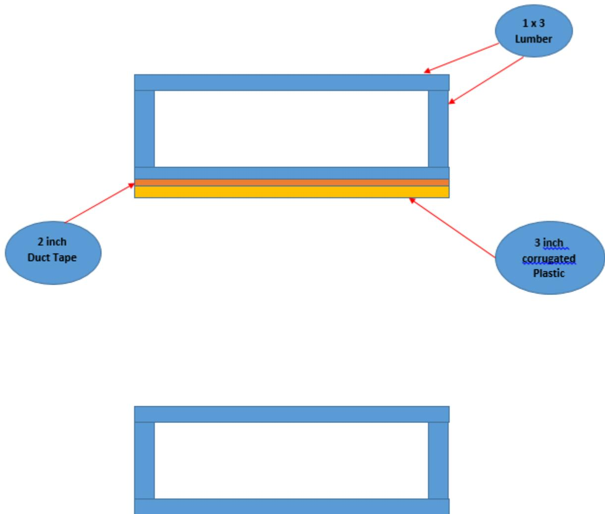
Cut to size the clear plastic sheet to fit over the whole wooden frame then staple to frame. Then using duct tape, tape the corrugated plastic to the wooden frame. The whole section should fit over 3 tanks. The plastic should be face down resting on the tanks. Some improvisation is need here. If there is a concern about using polyurethane, then use heavy duty Saran wrap (to wrap food with), which would be much cheaper.
