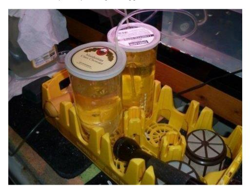
By using this set up, I can better control the temperature with a tank heater and can add additional bottles when needed.
